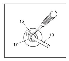
turn the Slotted Crank Nut counterclockwise until the arms are no longer loose. **Do not overtighten the Slotted Crank Nut.** When the Slotted Crank Nut is properly tightened, retighten the Crank Nut and reattach the left side shield.
